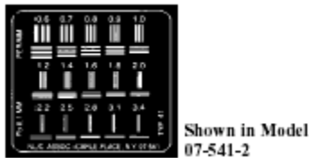
Fig 1. Spatial Resolution test patterns for Computed Radiography. 3
